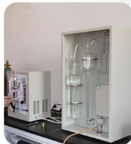
Carbon Sulfur Analyzer
