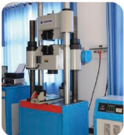
1000KN Electro-hydraulic Servo tensile Testing Machine
