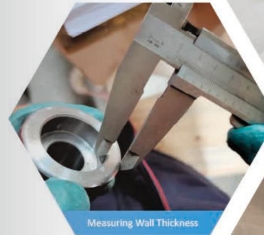
Measuring Wall Thickness
